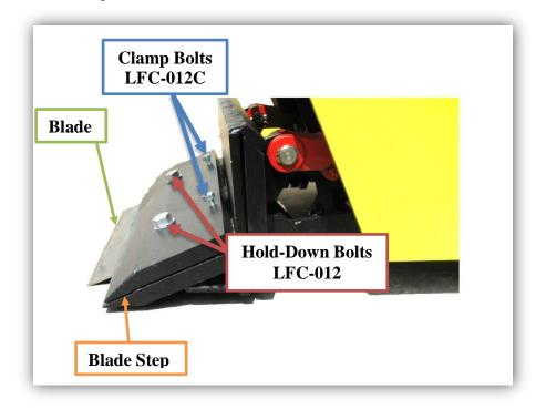
blades in 15 seconds. Dull blades may be sharpened and reused many times.
