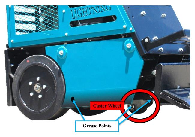
There are a 4 important grease points on the Lightning. A newer model Lightning will have a hole in the side weight cover for access to the grease zerk on the Lightning arms. If your Lightning does not have the access hole then simply remove the 2 bolts holding the side cover on for easy access. The other 2 points are on the caster assembly.
